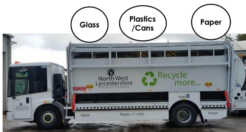
Figure 2-3: Side Kerbsider used by NWLDC
